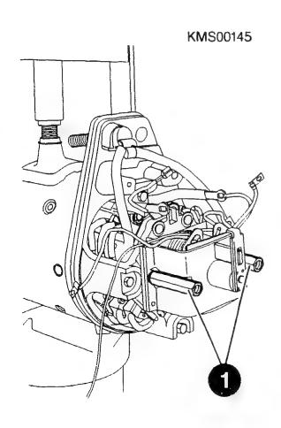
STARTING-MOTOR ASSEMBLY Assembling control relay and starting-motor solenoid Insert control relay with positioning pins in holes and secure with hexagon bolts (1). Use torque wrench. comm. avail. Torque wrench:
